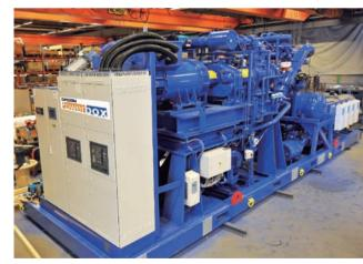
OPCON Powerbox ORC is suitable for low temperature hot water, steam and the other various hydrothermal fluid Working medium: liquid
