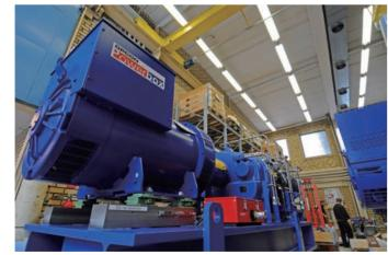
OPCON Powerbox WST is Suitable for high pressure dry or wet saturated steam and other high pressure gases
